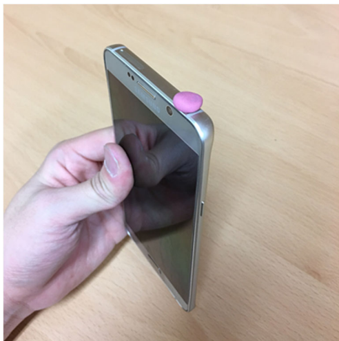
Fig. 13 Method of blocking microphone pinhole
